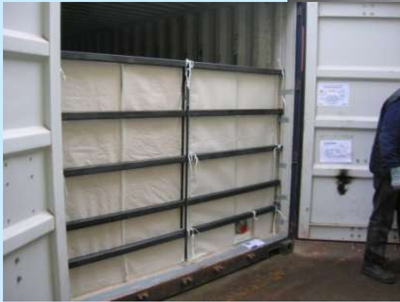
Bulkhead installation – bottom valve
